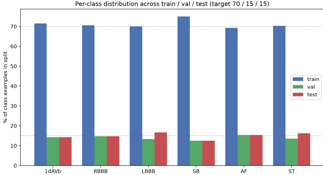
Figure 7. Per-class counts across train/validation/test splits. The multilabel-stratified split preserves class proportions within \pm 5\% of the nominal 70/15/15 ratio despite very small minority classes.
